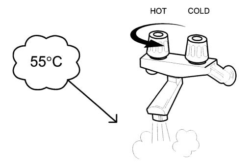
Rinnai Infinity water heaters without controllers are factory pre-set to a temperature limit of 55°C. Other limits, lower or higher, are available on request for the Infinity range. Temperature controllers are available that allow precise digital temperature control. Higher temperatures may be necessary for circulation loop systems.
